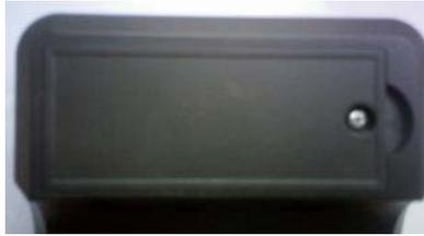
**Step2** Insert a 9V battery. There are anode and cathode marks in battery box and also a fixing tip. Reversely placed battery cannot be laid flat. Do not force the battery down, otherwise the battery box tip will be damaged.
