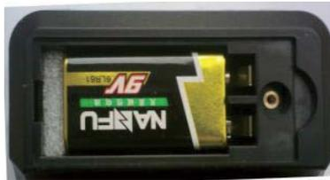
**Step3** Cover the battery box, and fix the screw.
