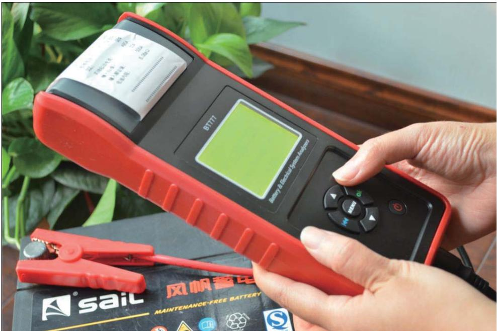
**BT777 Battery Tester with printer Manual Instruction (EN)**
